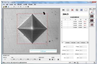
1, Easy Calibration, calibration can be done according to standard hardness blocks. Also can select calibration data according to test force, this function need to keep same test force with hardness tester.
